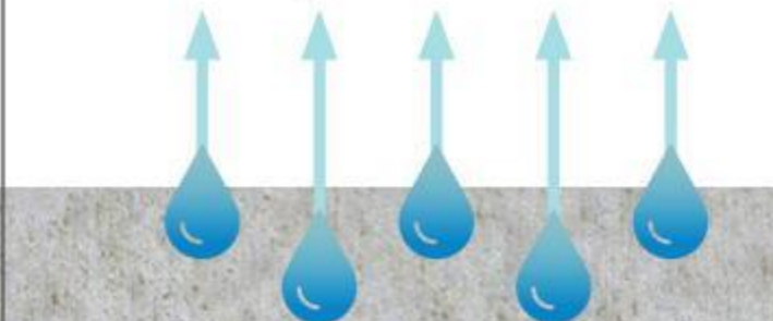
moisture moving out of concrete
