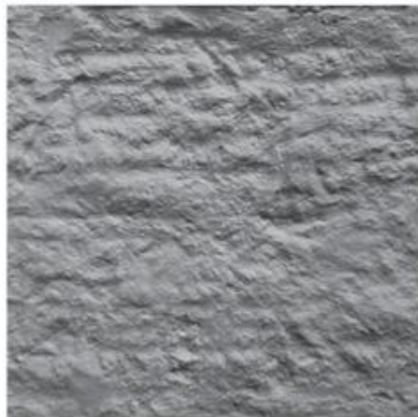
CSP 6 MEDIUM SCARIFICATION
