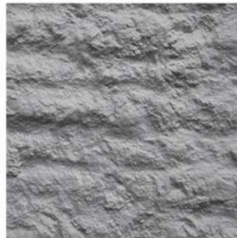
CSP 9 HEAVY SCARIFICATION
