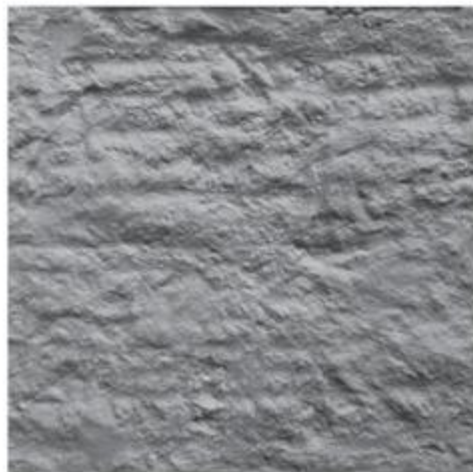
CSP 6 MEDIUM SCARIFICATION
